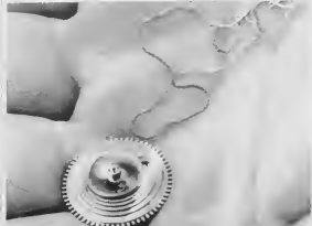
THE MINUTE hand-work which went into early watches is evidenced by this geared pulley "fusee" and chain. Made in individual links like a bicycle chain, it wrapped around the "fusee" and transmitted power from the mainspring. The gear teeth were hand-cut and filed to micrometer precision.
